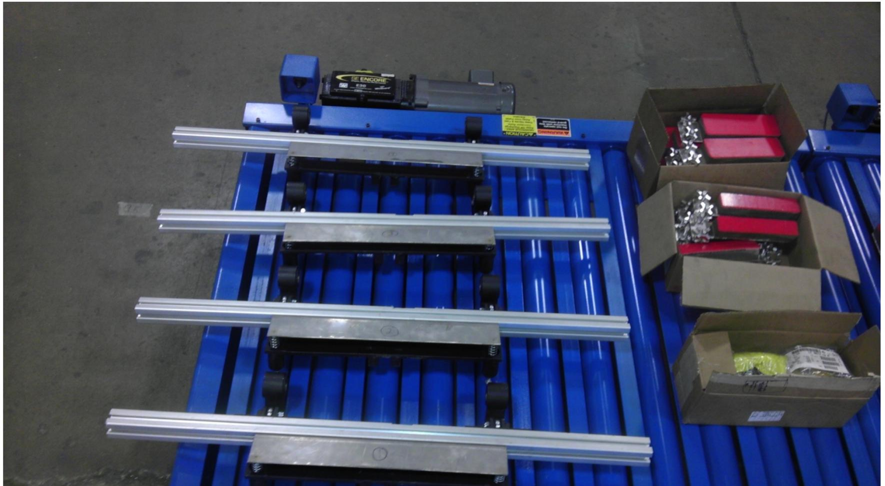
Install the new back stop assembly with the support pins, M10 bolts and washers
