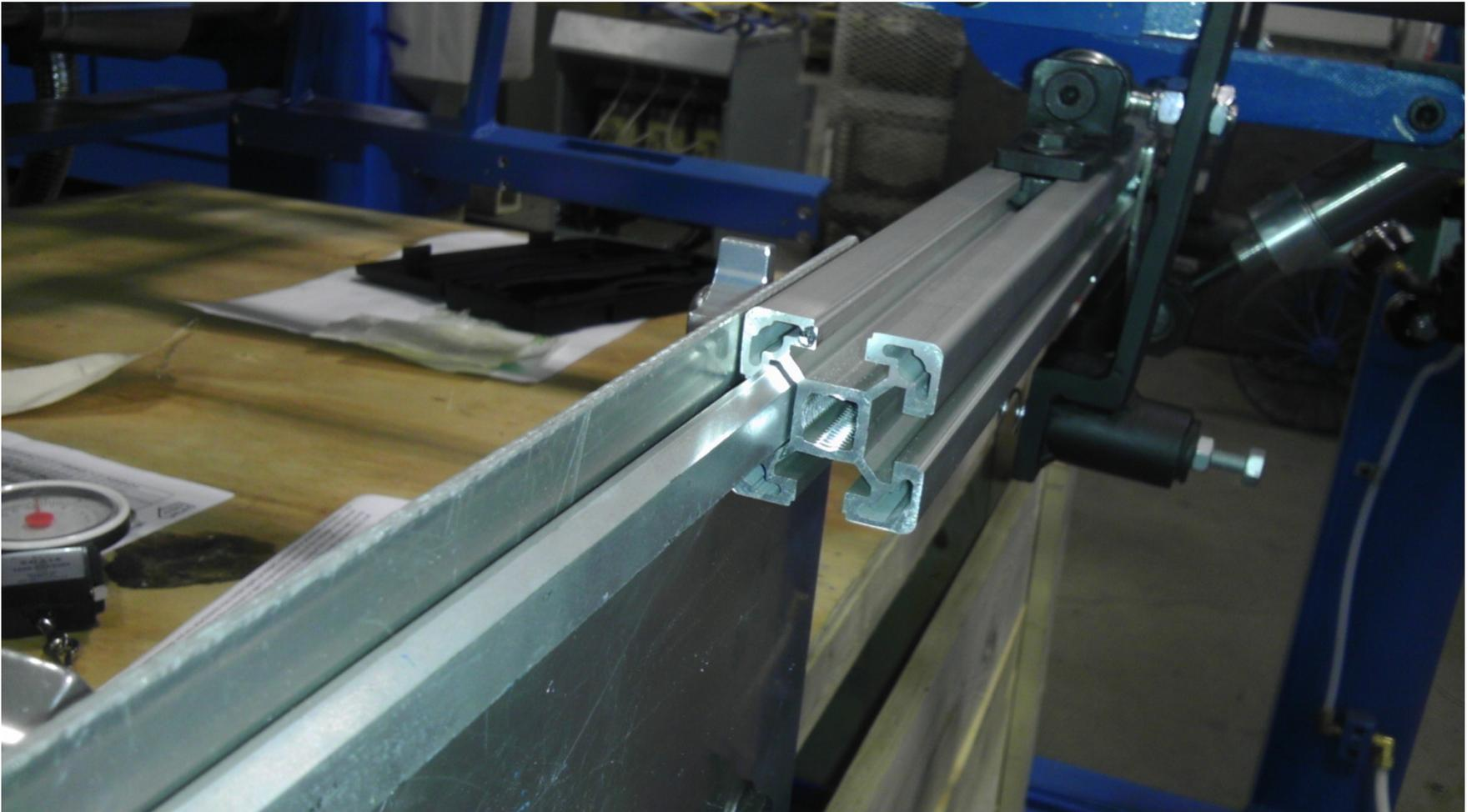
Use knobs to loosen and tighten the pads
